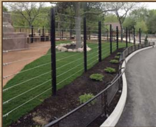
It took five layers of sturdy glass laminated with plastic to create the viewing window (left) into the hippo quarters. Space in the outdoor giraffe yard was expanded by using a fence with horizontal cables instead of a full moat. Skylights provide natural light for the giraffe indoor exhibit.
