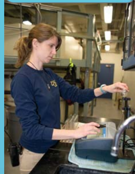
Uhlig tests the water in marine exhibits weekly with a spectrophotometer to make sure it doesn't contain toxic elements from fish waste.
